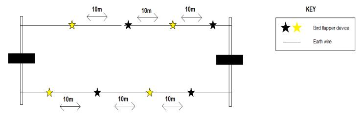
Technique and guideline for marking of the earth wire with bird flapper devices.
